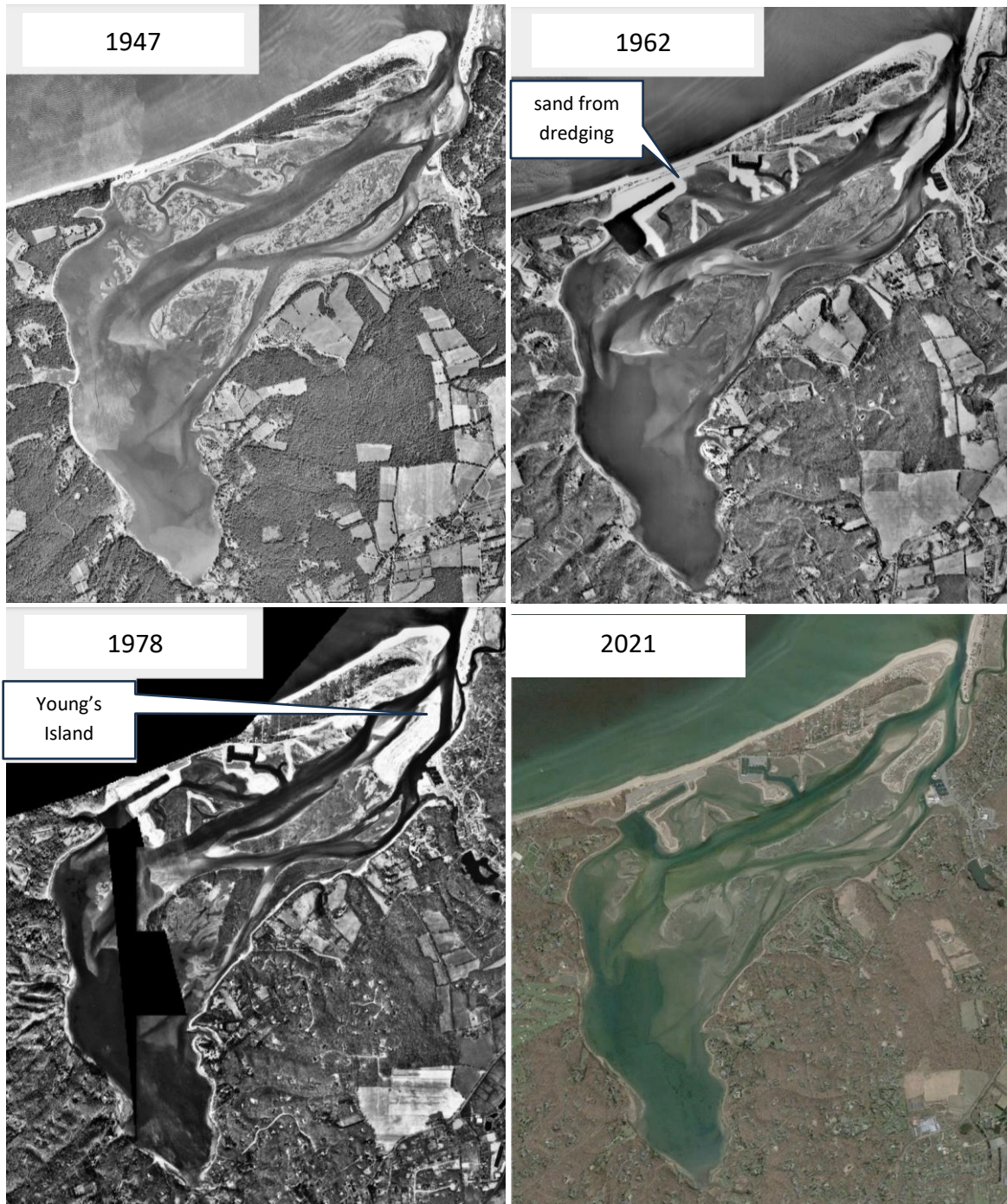
Figure 3. Historic Aerial Imagery of Stony Brook Harbor showing dredge spoil placement starting in 1962. (Suffolk County GIS, 2023)
