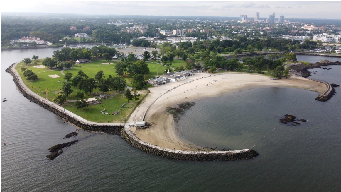
Figure 10. Glen Island Park photograph illustrating armored seawalls currently present (Source: Westchester County Parks Conservation Division, 2023)
