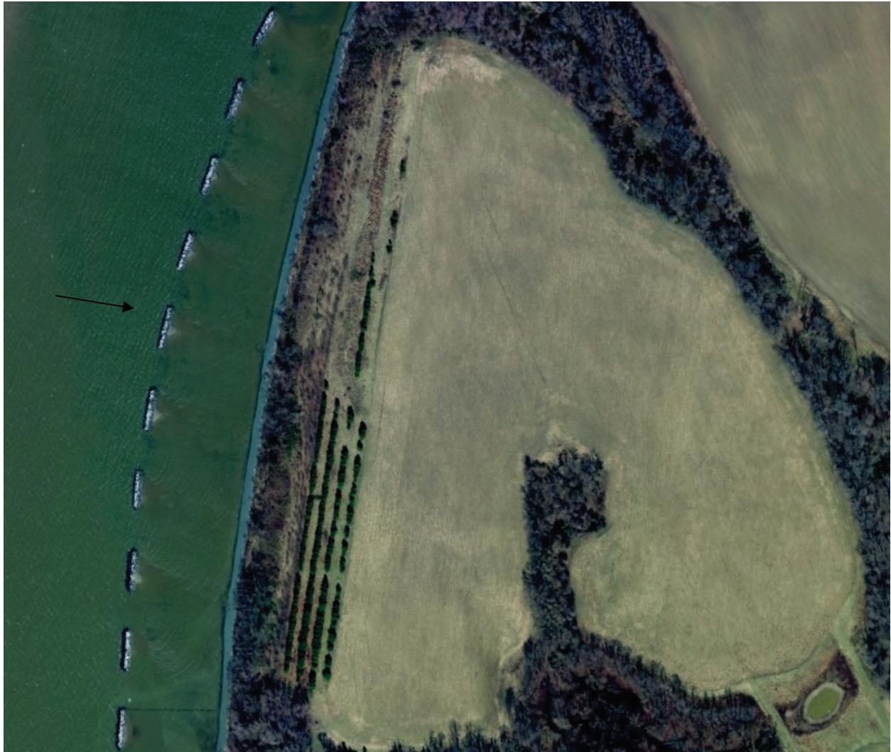
**Figure 3: Satellite Imagery of Offshore Breakwater in Northwestern Eastern Neck NWR.**
